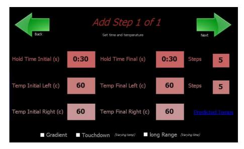
The 'Next' button will proceed through each of the parameter screens for each step contained within the cycling. After the parameters for each step are configured the operator is prompted to enter the number of times to repeat the cycle.
