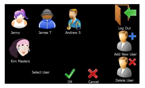
In the users area you are able to select an existing user or create or delete a user profile. When a user is selected Thermal profiles will be loaded or saved to a directory specific to that user. Logging out will change back to default user. To create a new user select the 'Add New User' icon and then enter the user name and select a user profile image.
