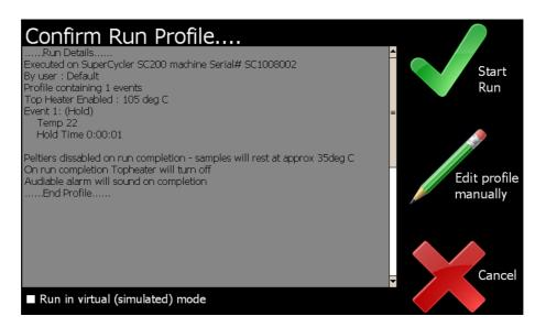
Once the run commences the software will automatically proceed to the 'Run' screen. You are not able to modify the profile once a run has commenced.
