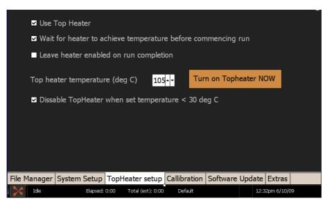
The following features are available under this tab for the top heater evaporation control:
